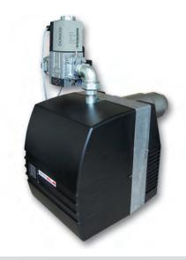
Fully automatic gas burner, tested and approved in accordance with DIN EN 676 suitable for the combustion of natural gas (-N) and liquefied gas (-F) in low-emission (version -LN) compliant with EN 676 Emission Class 3. Burner can be used horizontally and vertically.
